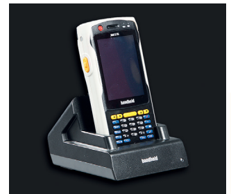
PDA Programmer Wireless two-way communication using a Windows based PDA with infra red port. Flash code, range and photocell switch level etc. can be set. With the Programmer also the event log can be retrieved.
