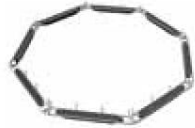
SEKİZGEN MONTAJ / OCTAGONAL MOUNTING İç Çap / Inner diameter: 965cm
